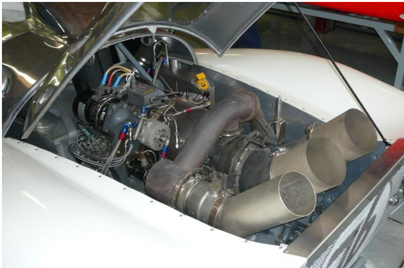
Le Howmet TX powered by a still-borne Continental TS325 (T65)
