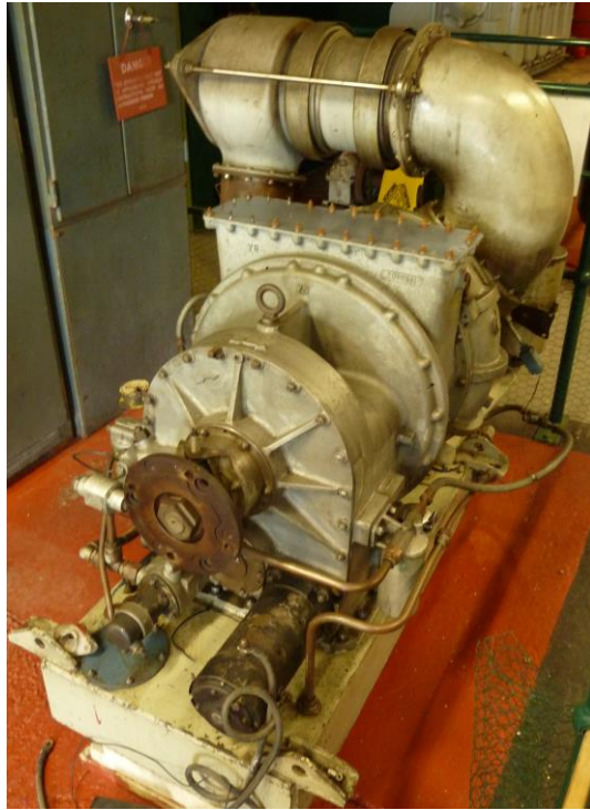
250HP stationary gas turbine built by the Austin Motor Company
