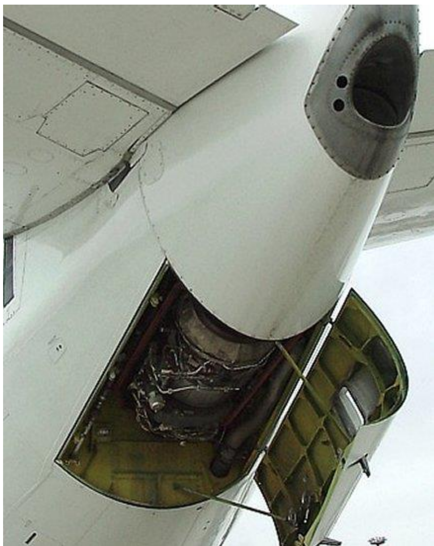
An installed aircraft gas turbine auxiliary power unit
