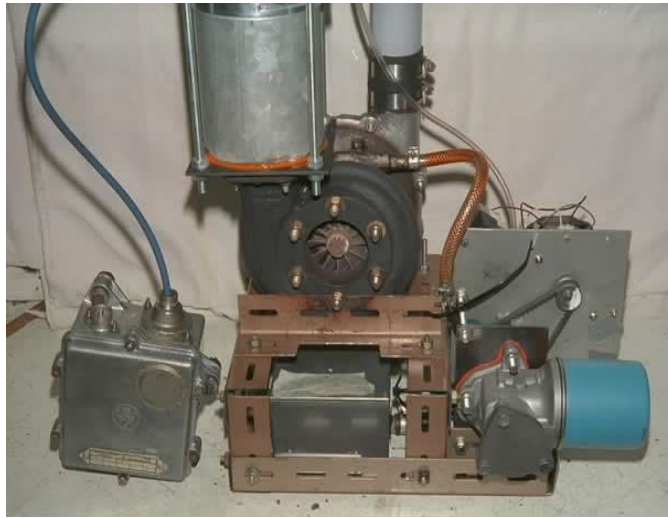
A homebuilt gas turbine engine utilizing an automotive turbocharger
